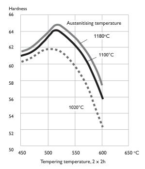
The tempering curves are obtained after heat treatment of samples with a size of  $15 \times 15 \times 40$  mm, cooling in forced air. Lower hardness can be expected after heat treatment of tools and dies due to factors like actual tool size and heat treatment parameters.
